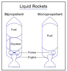
Fig. 5-7: Liquid Propellants
