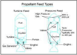
Fig. 5-8. Propellant Feed Types
