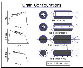
Fig. 5-10. Grain Configurations
