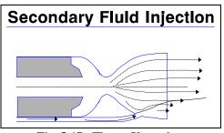
Fig. 5-17. Thrust Vectoring
