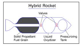
Fig. 5-11. Hybrid Rocket System
