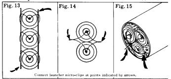
A combination of these two methods can be used for three engine circular clusters. First the engines are placed in the rocket so one igniter lead is toward the inside, the other toward the outside. The inner leads are twisted together. A wire loop (a large paper clip makes good raw material) is then formed and
