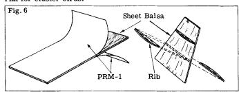
Fin stock thinner than 1/8" can be used, but it should be reinforced for best results. Two reinforcing methods are com-
