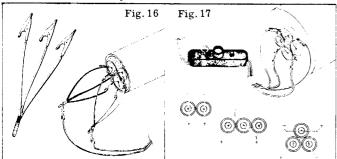
A variation of the clip whip system uses four micro-clips, permanently attached so two fork off from each launcher lead. The leads should be marked so the pairs of clips which are connected to the same lead can be easily identified. This system was developed for use with the four engine cluster in the Uprated Saturn I model, but also works well with two and three engine models. Fig. 17 illustrates a good four-clip electrical system along with several suggested connection methods.
