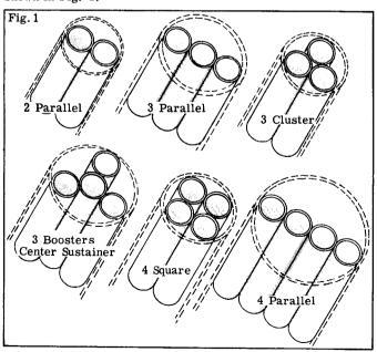
In designing a cluster rocket first make sure that thrust will be balanced around the center line of the rocket. An unbalanced arrangement will normally cause the rocket to veer off course. Similarly, all engines located away from the centerline of the rocket should develop the same amount of thrust. For example, the two outer engines in a parallel 3 engine cluster must be the same--although the center engine might be a B6-4, if one outer engine is a Bl4-5, the other one must be a Bl4-5.
