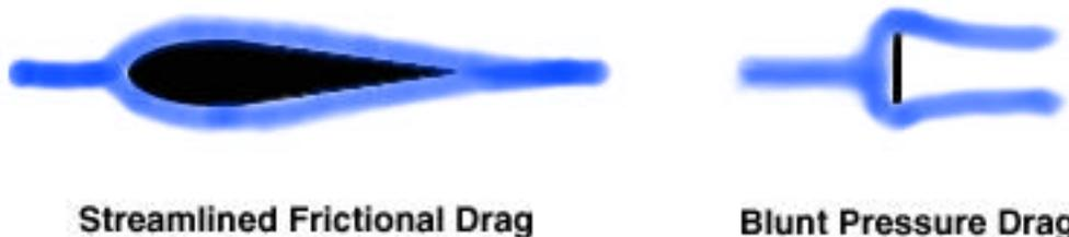
The propensity for frictional (viscous) and pressure drag to develop when fluid flows around a body depends on the body's shape, size, and surface characteristics. The actual magnitude of the drag will depend on the speed of fluid flow, and the properties of the fluid. The predominance of frictional or pressure effects will vary as the speed of the flow changes (a value called Reynolds Number provides a measure of what type of drag behavior to expect for a
