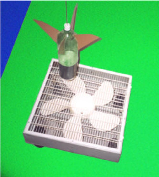
end of the string up to the scale and thread the string around the axle on the bottom end of the vertical post of the scale tray. Screw the cap onto a rocket you wish to test and suspend the rocket by the string above the scale. Adjust the distance the center of the front end of the water bottle (not the tip of a nose cone) hangs above the fan to be about 10 to 15 cm.
