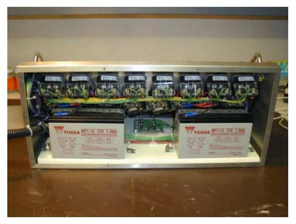
Inside view of console showing batteries
