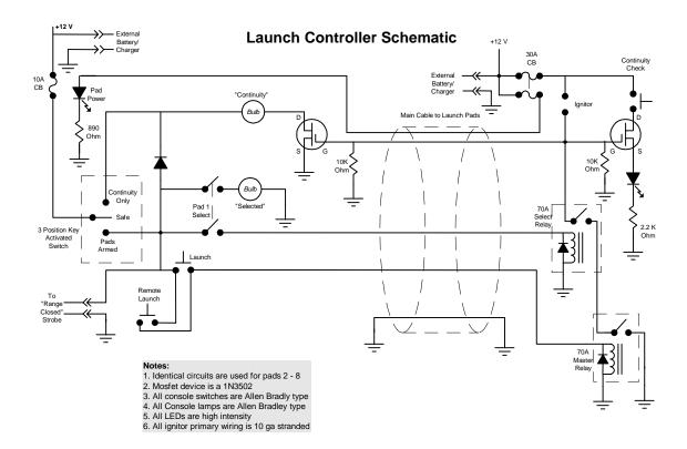
The pad side boxes contain two12v, 7Ah gel cell batteries wired in parallel and all internal wiring is 10 ga stranded copper wire. The connections to the pads are 14 ga stranded wiring with typical copper clips soldered to the ends. A 30A circuit breaker protects the pad boxes in the event of an overload condition.
