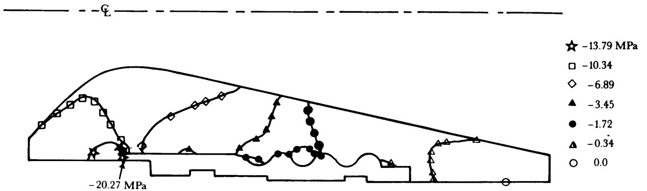
Figure 7-51. Minimum Principal Stress Contours
