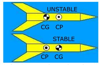
forward. Because of this action, the rocket is pointed into the relative wind.
