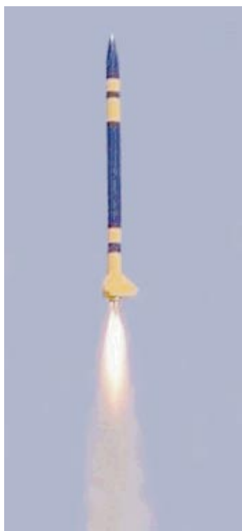
My scratchbuilt 329 was one of my favorite rockets to have fun with, having 3 x 29mm motor mounts in a 3" diameter airframe. I have flown it on all sorts of motors, ranging from F25s all the way up to G125s. This photo shows three G40 White Lightning motors powering it to an altitude of 3000 feet.
