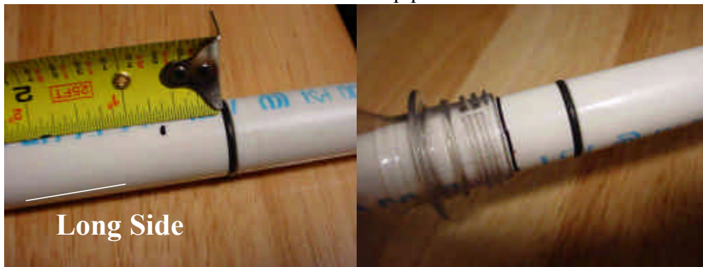
Figure 6. Drawing cable tie alignment line.
