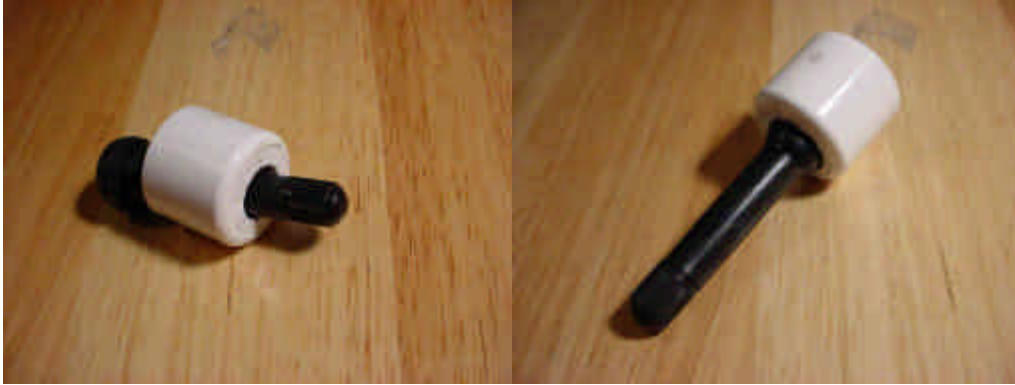
Figure 3. Pressing in the valve.
