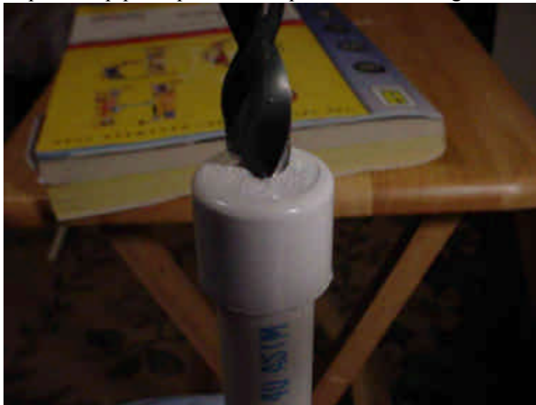
Figure 2. Drilling the valve hole.
