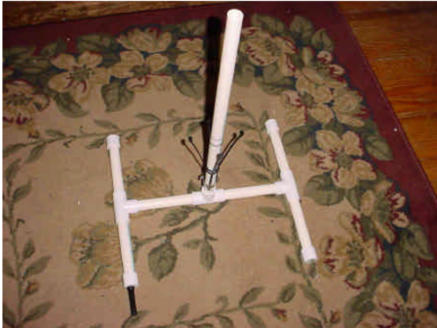
Figure 9. Launcher assembly after joints are cemented.
