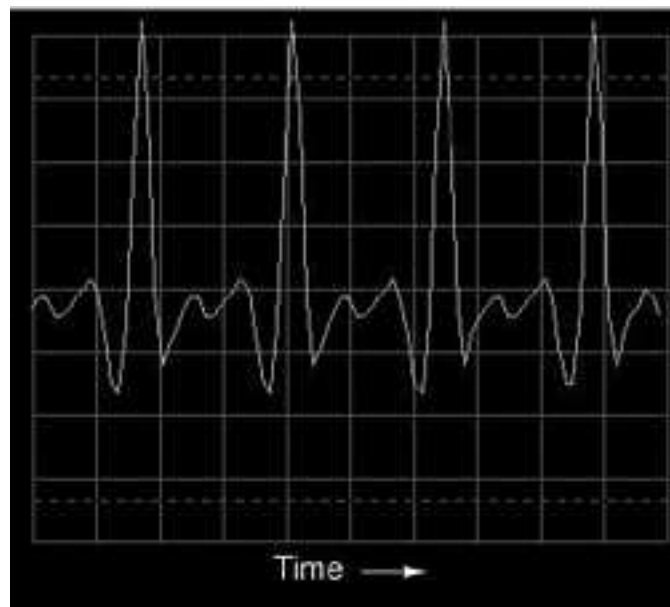
Figure 7.27: Oscilloscope display: waveshape of a trumpet tone.
