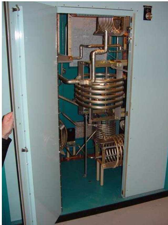
Figure 3.18: High power inductors formed from hollow tubes.
