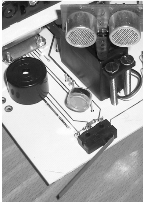
Figure 8.12 Some of Derbot's sensors and actuators – an ultrasonic distance sensor mounted on a Futaba servo, behind a light-dependent resistor and microswitch
