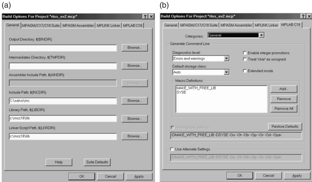
Figure 19.5 Setting build options for Salvo. (a) General. (b) MPLAB C18
