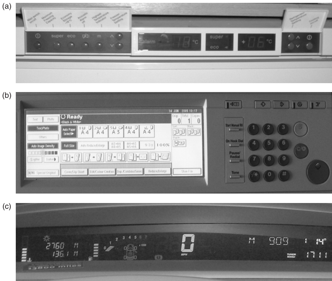
Figure 8.1 The human interface in some familiar products. (a) Domestic fridge. (b) Photocopier. (c) Car dashboard (detail)
