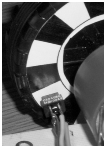
Figure 8.15 A reflective opto-sensor used as a shaft encoder on the Derbot
