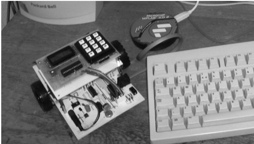
Figure 7.21 ICD 2 connected to a Derbot AGV
