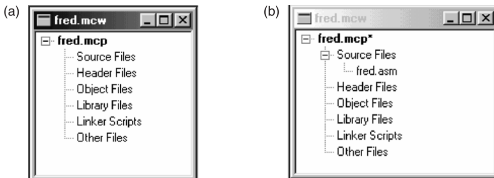
Figure 4.7 Workspace window. (a) For a newly created project. (b) For a project with source file added
