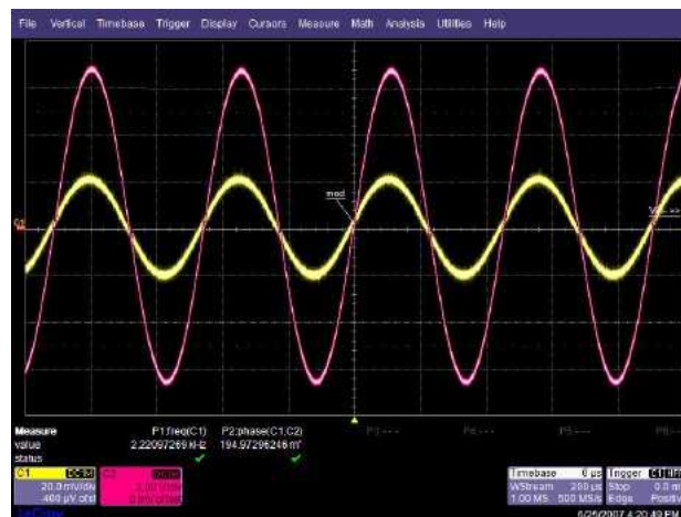
Figure 8.3: OPA227 A_v=50\text{dB} @ 2.2 kHz
