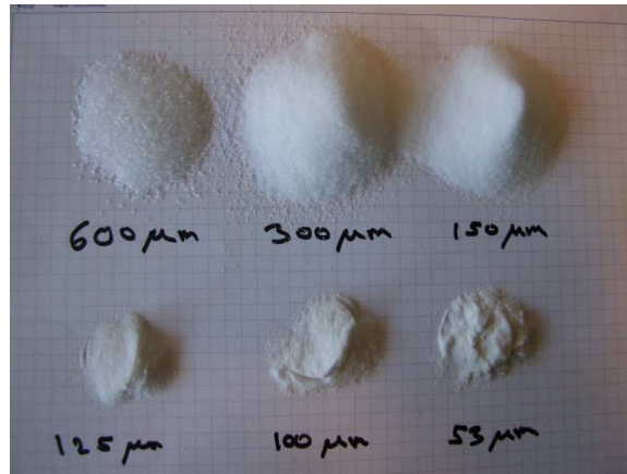
Figure 6.1: Sieved particles showing the particle distribution. Note that the markings indicates the particle size that was retained on each screen.
