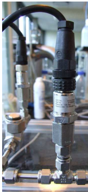
Figure 6.19: Pressure transducers for recording pressure during strands firing. Particle filter in between.
