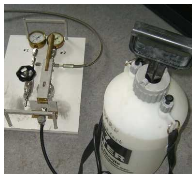
Figure 6.12: Hydraulic piston pump used for hydrostatic tests.
