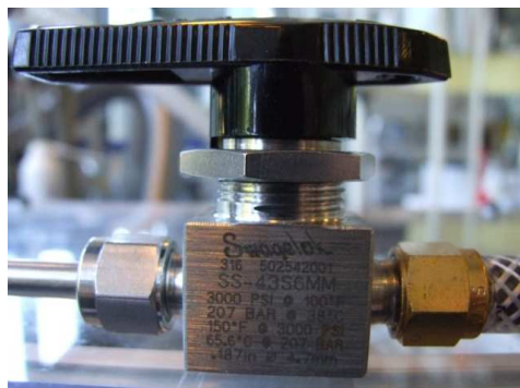
Figure 6.22: Ball valve for releasing of nitrogen and combustion gases.
