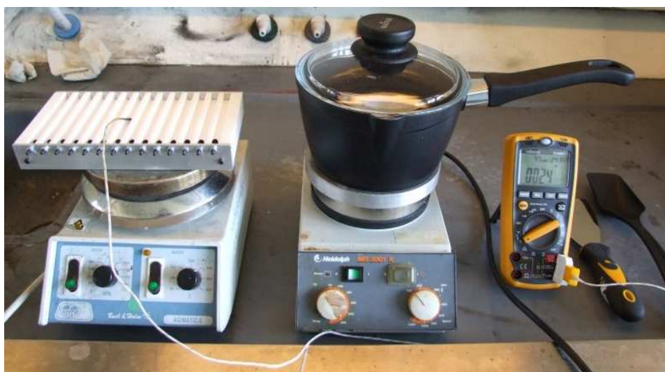
Figure 6.4: From left to right: Casting mold prior to heating on a hot plate, PTFE coated pot with sorbitol based propellant and a multimeter for measuring mold and slurry temperature as well as relative humidity.
