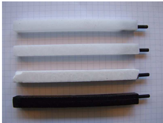
Figure 6.6: From top to bottom: Strands of fully cured KN-Sorbitol, KN-Erythritol, KN-Mannitol and painted KN-Erythritol.
