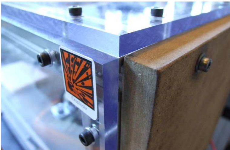
Figure 6.23: Structural frame where the polycarbonate and MDF plates are connected to the aluminum strut profiles.
