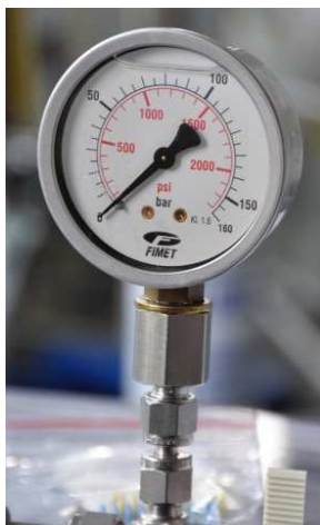
Figure 6.20: Pressure gauge for visual inspection of firing vessel pressure.
