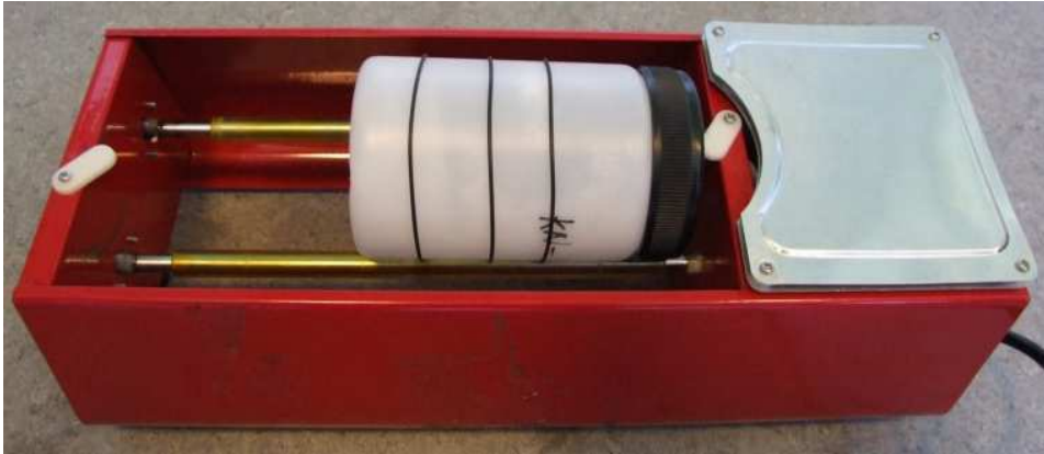
Figure 6.2: Polyethylene jar and ball mill.
