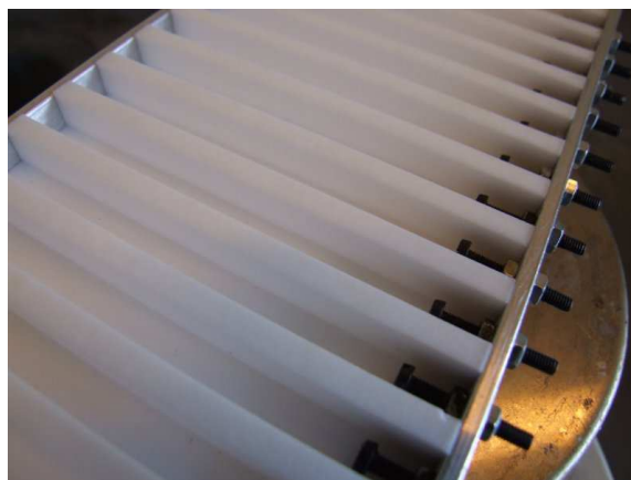
Figure 6.3: PTFE casting mold with 8x8 mm grooves for propellant and M3x20 bolts for attachment to the strand holder.
