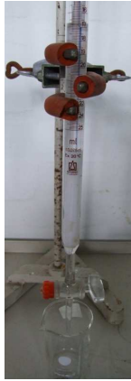
Figure 6.7: KN-Sorbitol immersed in ethanol in a burette.
