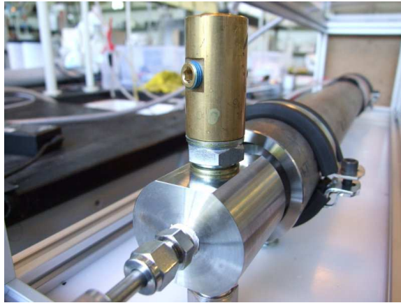
Figure 6.16: Burst disc housing with nickel diaphragm.
