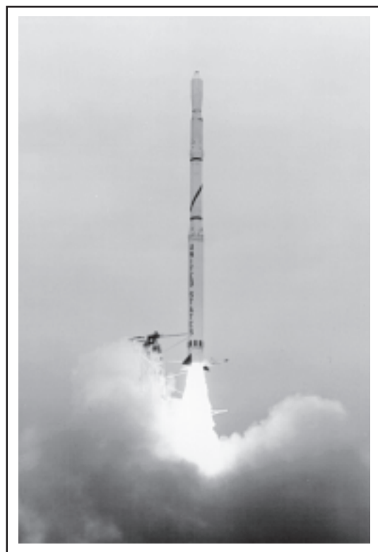
NASA's Scout rocket is a four-stage solid rocket booster that can launch small satellites into Earth orbit. The Scout can carry about a 140 kilogram payload to a 185 kilometer high orbit. NASA used the Scout for more than 30 years. This 1965 launch carried the Explorer 27 scientific satellite.
