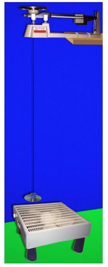
Solve the drag equation (Eq 1) for velocity to obtain (Eq 2). Use the calculated drag force, known drag coefficient (C<sub>d</sub> =1.17), and CD area in Eq 2 to get an apparent air velocity  $V(m/s^2)^{**}$
