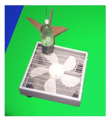
end of the string up to the scale and thread the string around the axle on the bottom end of the vertical post of the scale tray. Screw the cap onto a rocket you wish to test and suspend the rocket by the string above the scale. Adjust the distance the center of the front end of the water bottle (not the tip of a nose cone) hangs above the fan to be about 10 to 15 cm.
