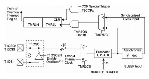
Figure 2.33: Block diagram of Timer 3
