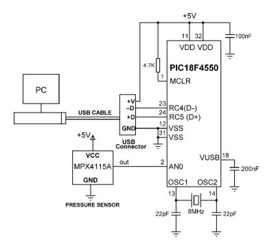
Figure 8.37: Circuit diagram of the project
