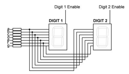
Figure 6.29: Two multiplexed 7-segment displays
