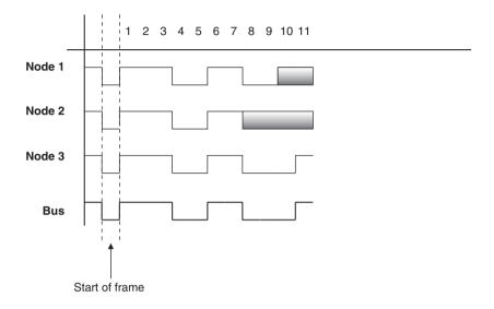
Figure 9.9: Example CAN bus arbitration
