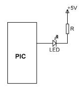
Figure 4.14: Connecting the LED in current sinking mode
