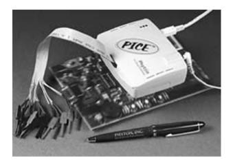
Figure 5.23: PICE-MC in-circuit emulator
