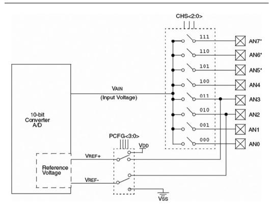
Figure 2.41: Block diagram of the PIC18F452 A/D converter
