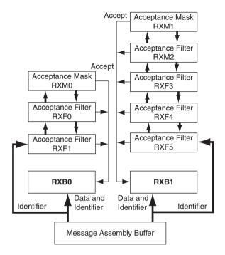
Figure 9.13: Receive buffer block diagram
