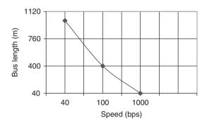
Figure 9.4: CAN bus speed and bus length
