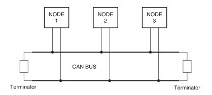
Figure 9.2: Example CAN bus
