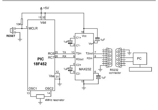
Figure 6.54: Circuit diagram of the project
