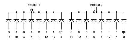
Figure 6.30: DC56-11EWA display segment configuration
