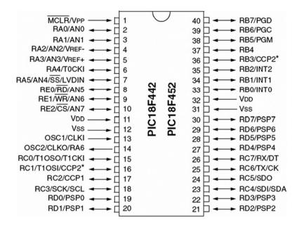
Figure 2.1: PIC18F452 microcontroller DIP pin configuration
