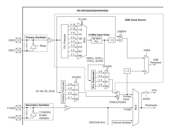
Figure 8.23: PIC18F4550 microcontroller clock
