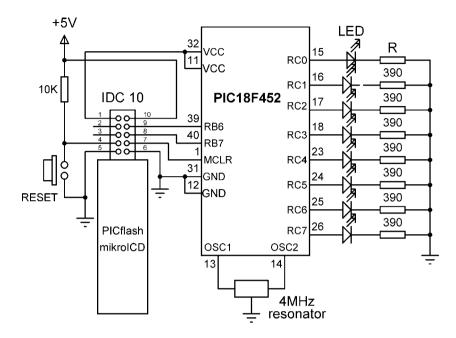
Figure 5.50: Circuit diagram of the project
