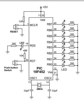
Figure 10.10: Circuit diagram of the project
