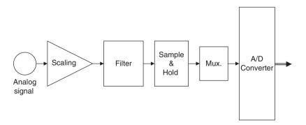
Figure 2.40: Signal conditioning and A/D conversion process
