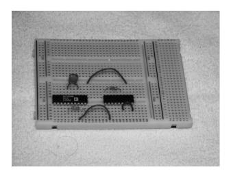
Figure 5.26: Picture of a breadboard with some components
