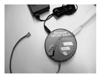
Figure 5.17: ICD2 in-circuit debugger
