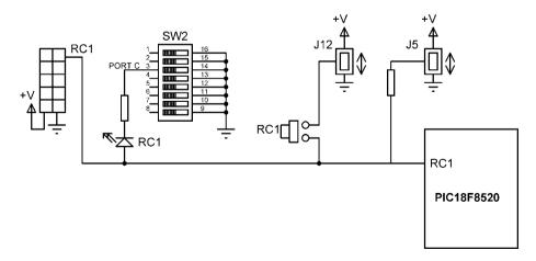
Figure 5.58: LED and push-button switch connections
