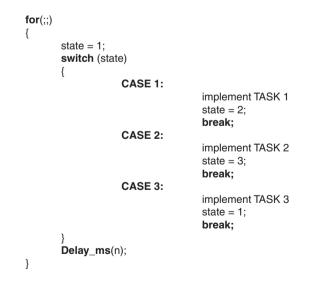
Figure 10.3: Selecting the next state from the current state
