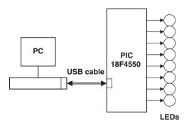
Figure 8.10: Block diagram of the project
