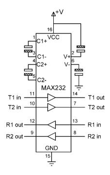
Figure 6.52: MAX232 pin configuration
