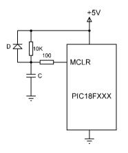
Figure 2.12: Reset circuit for slow-rising voltages
