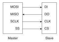
Figure 7.3: SPI master-slave connection
