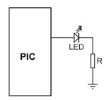
Figure 4.15: Connecting the LED in current sourcing mode
