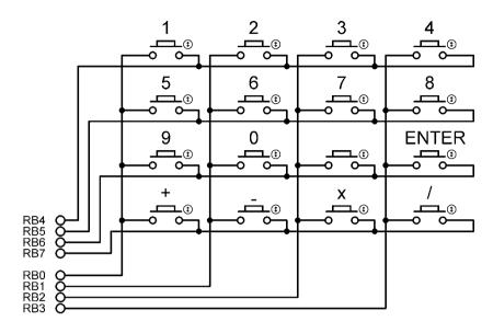
Figure 6.44:  $4 \times 4$  keypad structure
