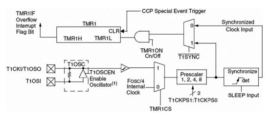
Figure 2.28: Internal structure of Timer 1
