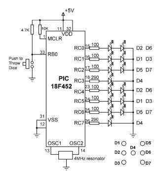
Figure 6.16: Circuit diagram of the project
