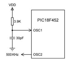
Figure 2.19: 2MHz clock in RC mode
