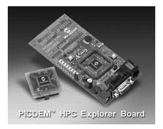
Figure 5.4: PICDEM HPC Explorer development board
