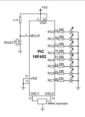
Figure 6.3: Circuit diagram of the project
