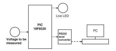
Figure 10.12: Block diagram of the project
