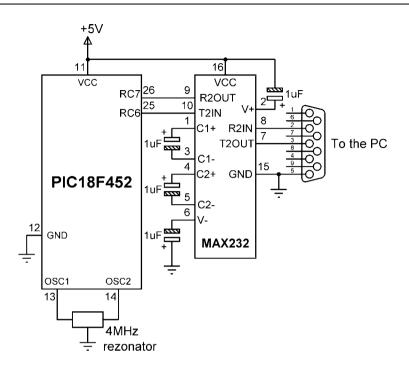
Figure 4.25: Circuit diagram of Example 4.14
