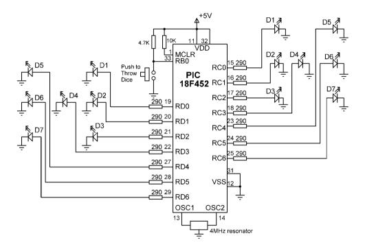
Figure 6.13: Circuit diagram of the project
