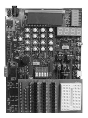
Figure 5.5: MK-1 Universal PIC development board
