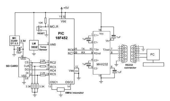
Figure 7.14: Circuit diagram of the project
