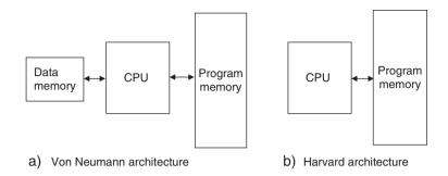
Figure 1.4: Von Neumann and Harvard architectures
