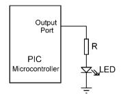
Figure 6.2: LED connected in current sourcing mode
