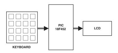
Figure 6.45: Block diagram of the project
