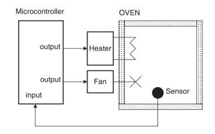
Figure 1.1: Microcontroller-based oven temperature control system
