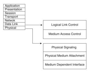
Figure 9.6: CAN and the OSI model
