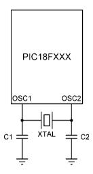
Figure 2.14: Using a crystal as the clock input
