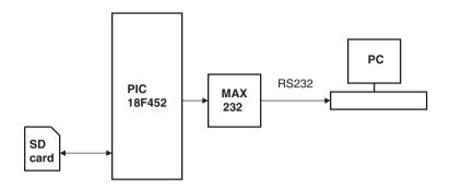
Figure 7.7: Block diagram of the project
