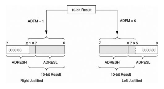
Figure 2.44: Formatting the A/D conversion result
