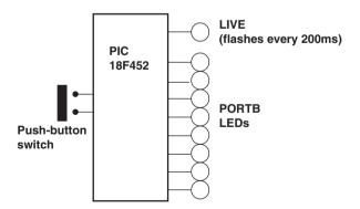
Figure 10.9: Block diagram of the project
