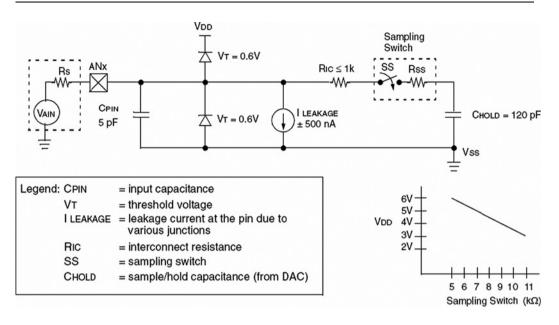
Figure 2.45: Analog input model of the A/D converter
