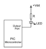
Figure 6.1: LED connected in current sinking mode
