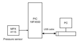
Figure 8.36: Block diagram of the project
