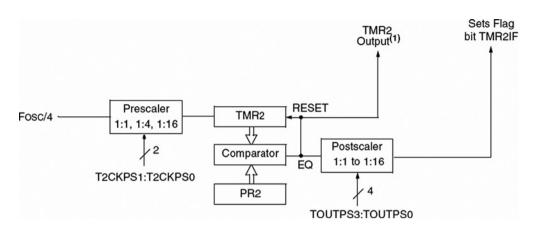
Figure 2.31: Timer 2 block diagram
