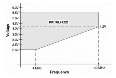
Figure 2.10: Operation of PIC18LF452 at different voltages
