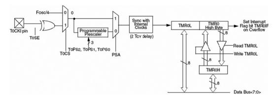
Figure 2.26: Timer 0 in 16-bit mode
