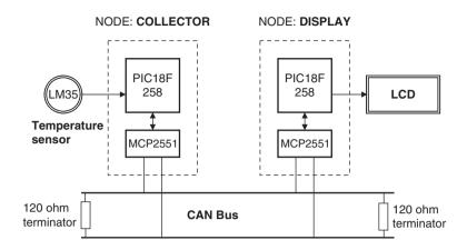
Figure 9.15: Block diagram of the project
