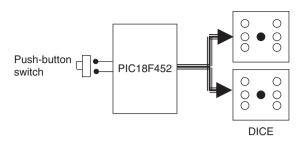
Figure 6.12: Block diagram of the project
