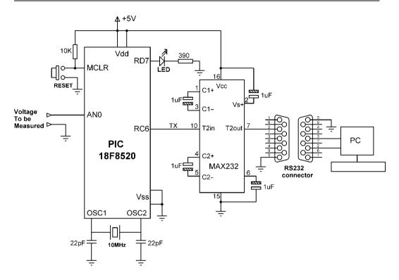
Figure 10.13: Circuit diagram of the project
