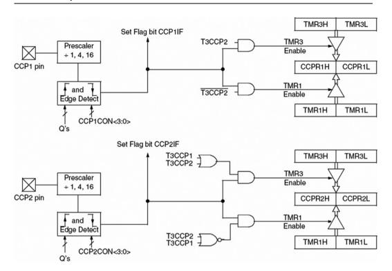
Figure 2.35: Capture mode of operation
