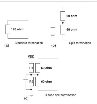
Figure 9.5: Bus termination methods
