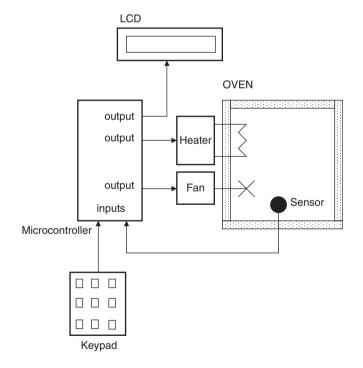
Figure 1.2: Temperature control system with a keypad and LCD
