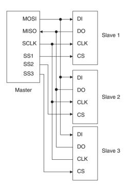
Figure 7.4: Multiple-slave SPI bus
