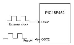
Figure 2.17: External clock in EC mode
