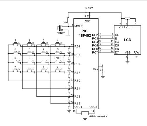
Figure 6.46: Circuit diagram of the project
