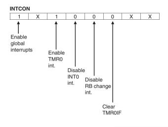
Taking the don't-care entries (X) as 0, the hexadecimal value to be loaded into register INTCON is  $0 \times A0$ .
