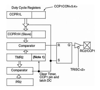
Figure 2.38: PWM module block diagram
