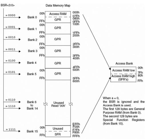
When a = 1, the BSR is used to specify the RAM location that the instruction uses.
