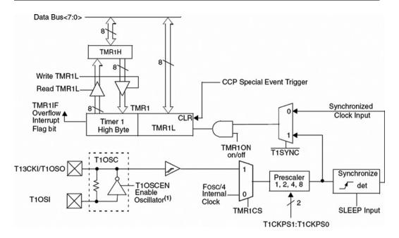
Figure 2.29: Timer 1 in 16-bit mode
