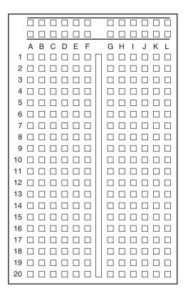
Figure 5.24: A typical breadboard layout
