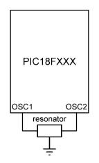
Figure 2.15: Using a resonator as the clock input
