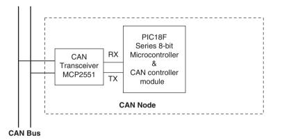
Figure 9.12: CAN node with integrated CAN module
