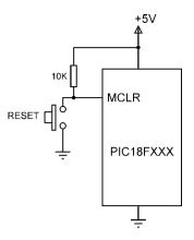
Figure 2.13: External reset circuit
