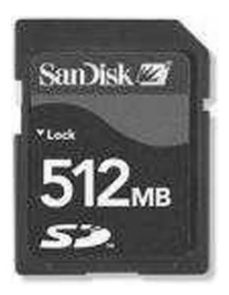
Figure 7.1: A typical SD card
