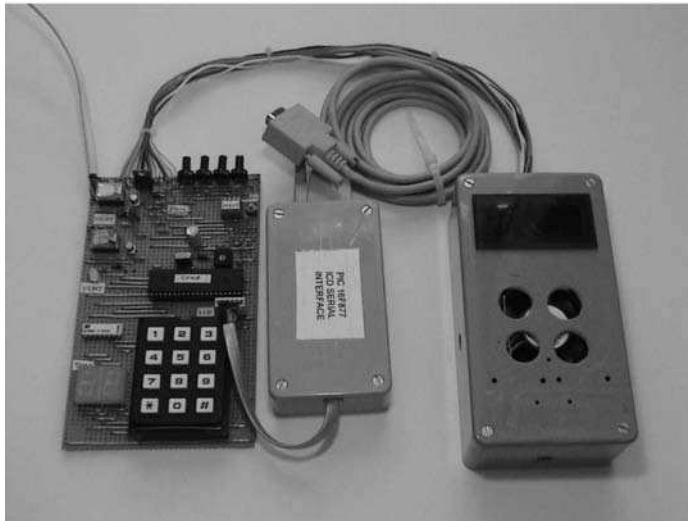
Figure 15.6 TEMPCON system. (a) Stripboard version of temperature controller board; (b) Temperature controller system with ICD module and dummy load.
