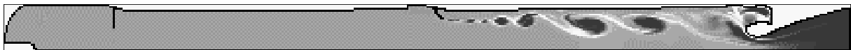
Figure 9: Computation of the Coupling between Vortex-Shedding and Two-Phase Flow in an Unstable Segmented Solid Rocket Motor (Particles Volume Fraction).
