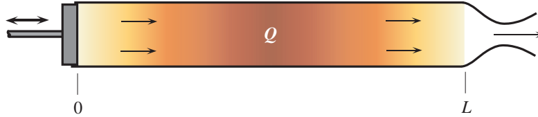
FIGURE 6.1. A Tube with Distributed Heat Addition and an Oscillating Piston to Drive Waves
