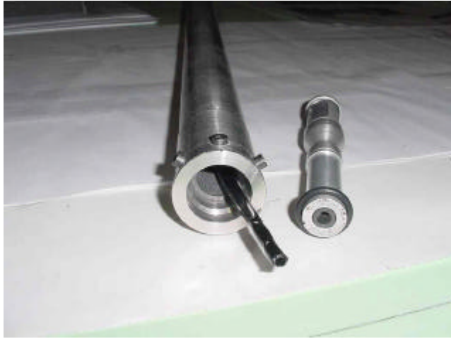
Photo 6. MECH_FA_01 Microhybrid motor. The motor is presented together with 38 mm Hybrid motor for scalling.
