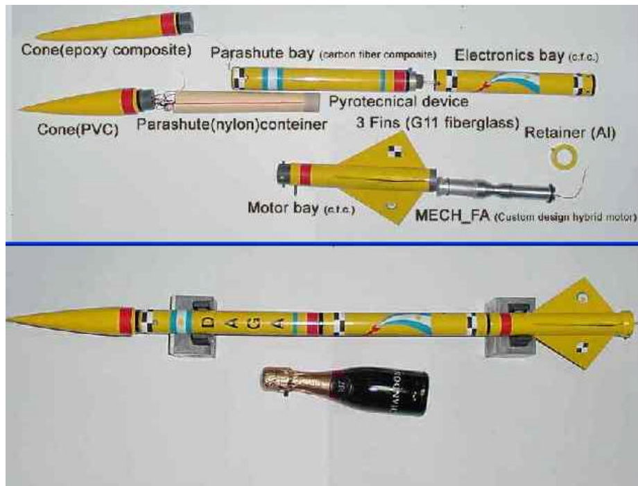
Photo 2. DAGA_MECH_FA_01 Microhybrid Rocket. The rocket's parts and armed rocket presentation. Bottle (little) of Chandon Champagne is seated for scale.
