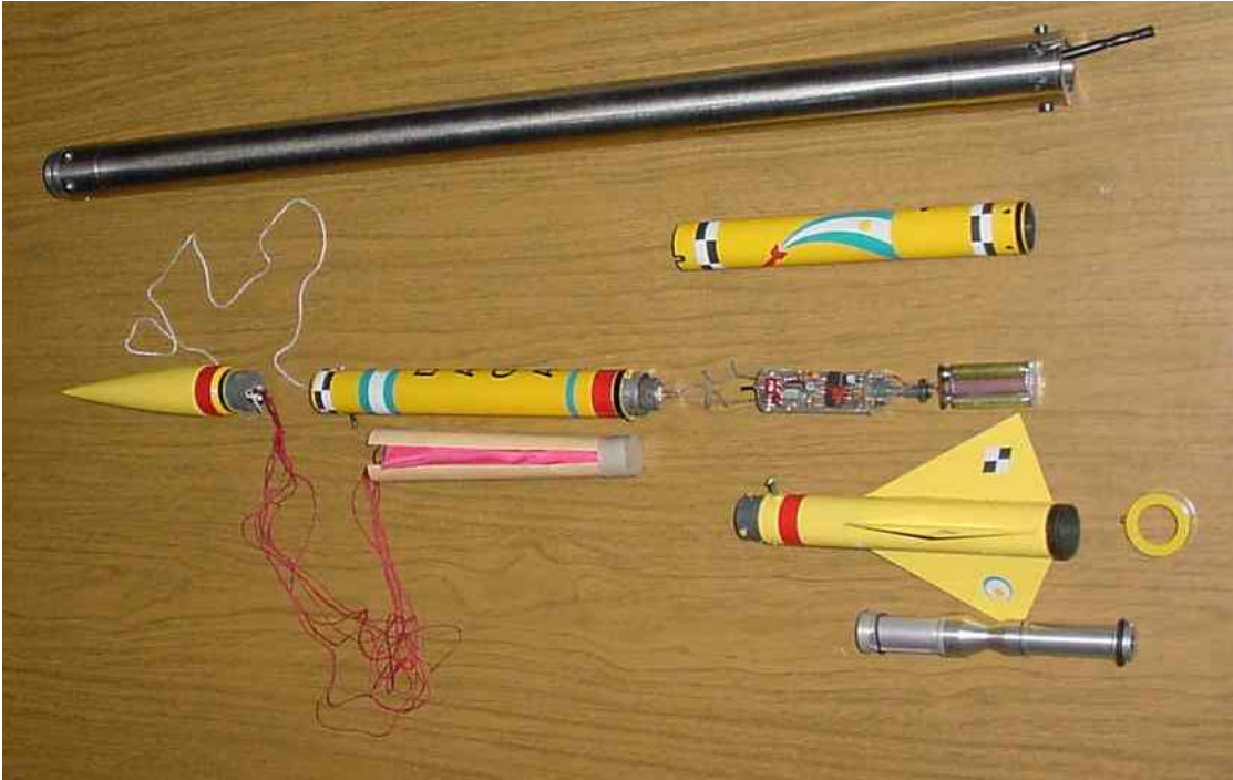
Photo 3. DAGA_MECH_FA_01 Microhybrid Rocket. After flight test 16.02.05. 38 mm - Monocock hybrid Urbansky-Colburn motor is for scale.
