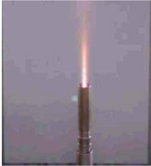
Photo 8. MECH_FA_01 Microhybrid motor: the photo depicts of the “mach diamonds” in the exhaust plume.
