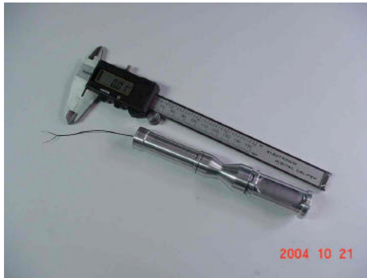
Photo 5. MECH_FA_01 Microhybrid motor.
