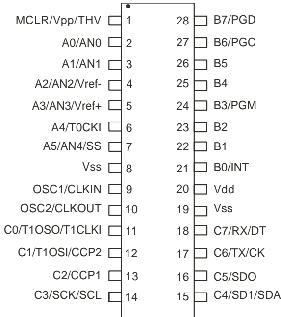
Figure 16.1 The 16F870/2/3/6 pinout
