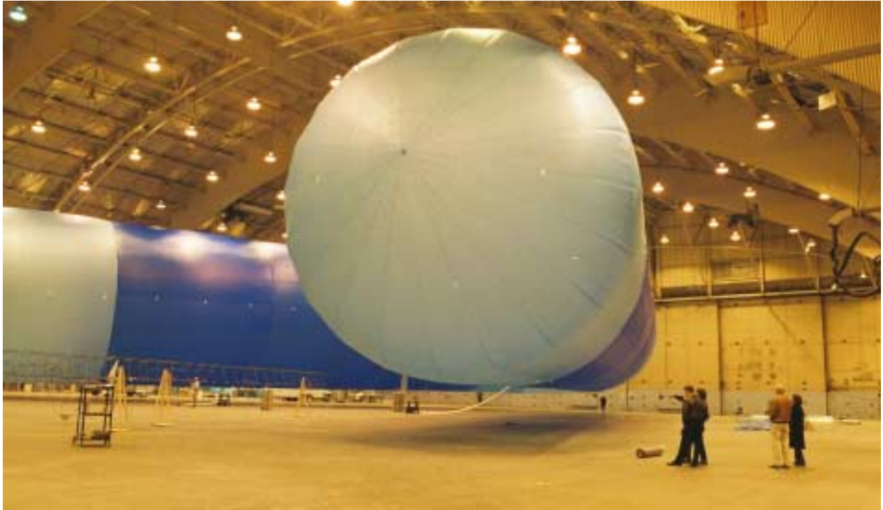
175 foot long Ascender float test.
