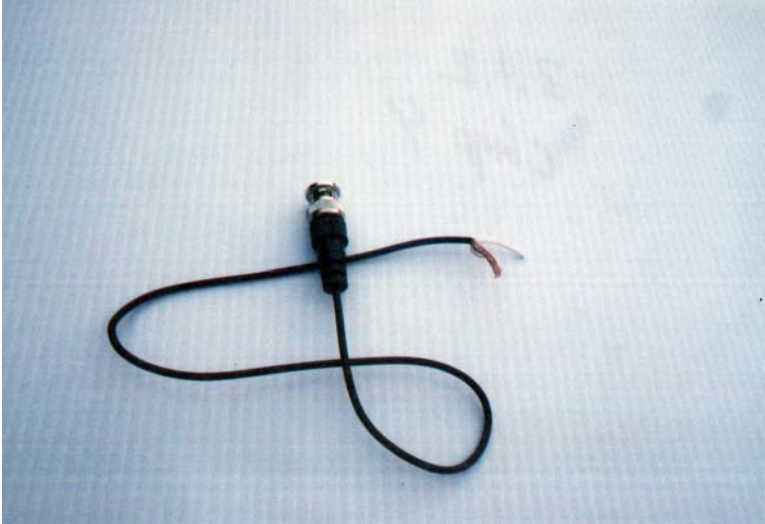
Stripped RG-174 - The coax cable with the center conductor pulled through the outer braided jacket.
