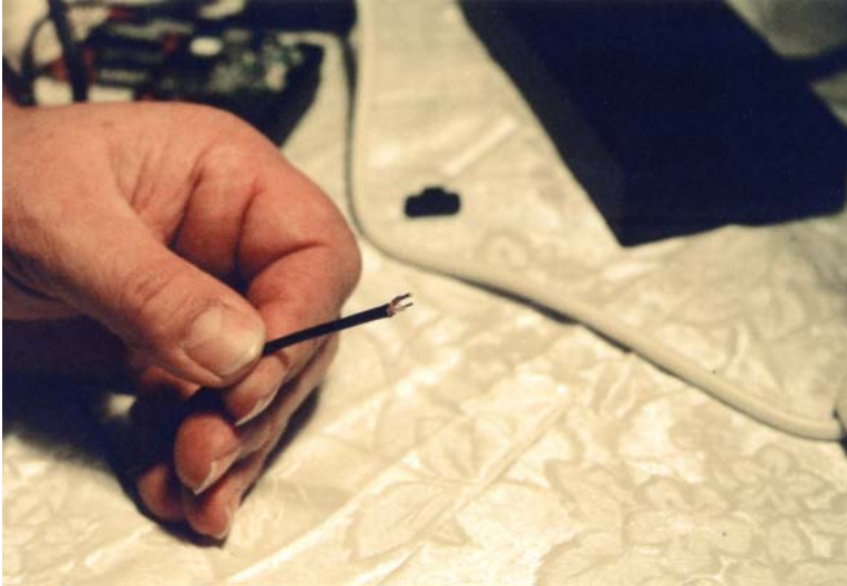
Making the Antenna - The cut and stripped RG-174 coax.
