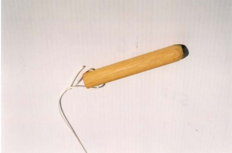
Release Pin - Round the end to help prevent snagging.
