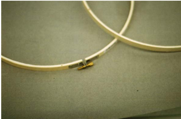
A needle point ring before it is converted into a parachute ring. Opened ring shows the clamp and rivets
