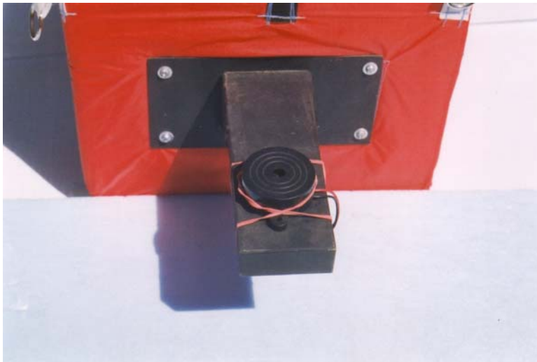
Place the audio beacon securely on a boom.
