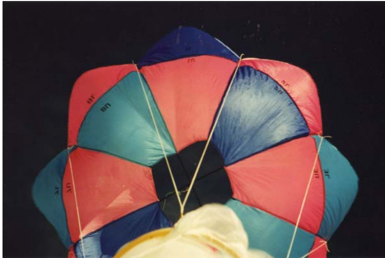
After balloon burst - The parachute shortly after balloon burst. It appears that some of the balloon remains are wrapped around the parachute ring. At this point, descent speed is around 100 mph!
