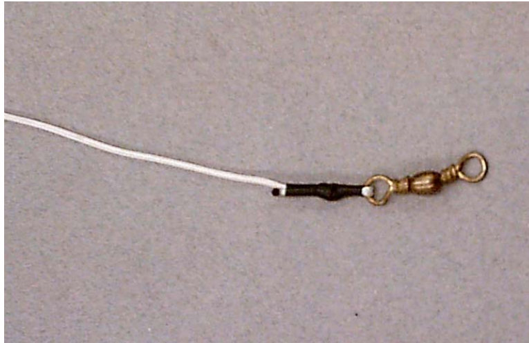
Heat Shrink Tubing – Securing the knot.
