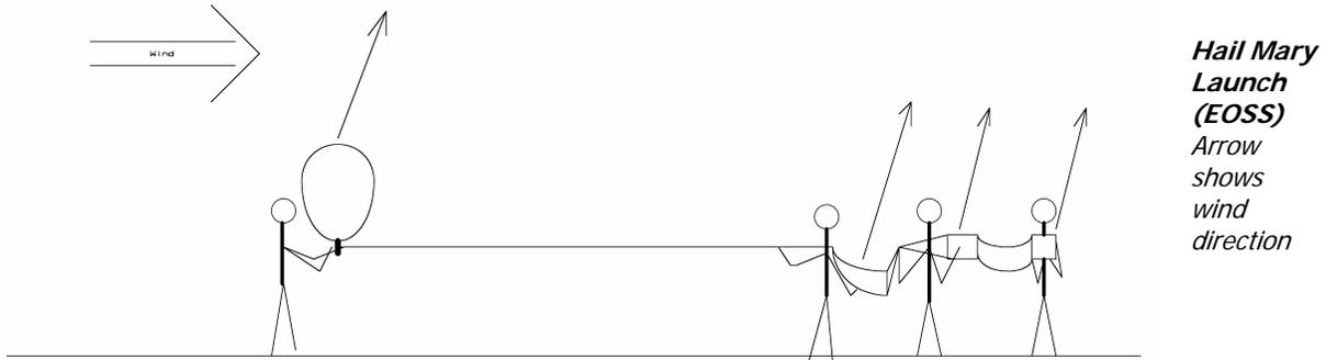
TVNSP has used this method to launch in high surface winds. The stack was released in the wind shadow of a building.
