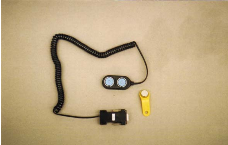
A ThermoChron Kit - The reader cable plugs into a serial port. The thermoChron is the silver disk inside the plastic fob.
