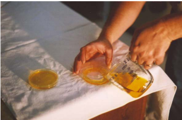
Pouring Agar - Quickly lift the lid of the sterile petri dish and pour the hot, liquid agar.
