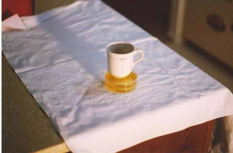
A stack of petri dishes cooling- A mug of hot water on top of the dishes reduces the condensation inside the petri dishes.
