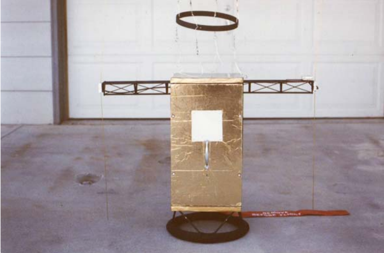
The Isaac Asimov - My first near spacecraft. Note the truss structure of the booms.
