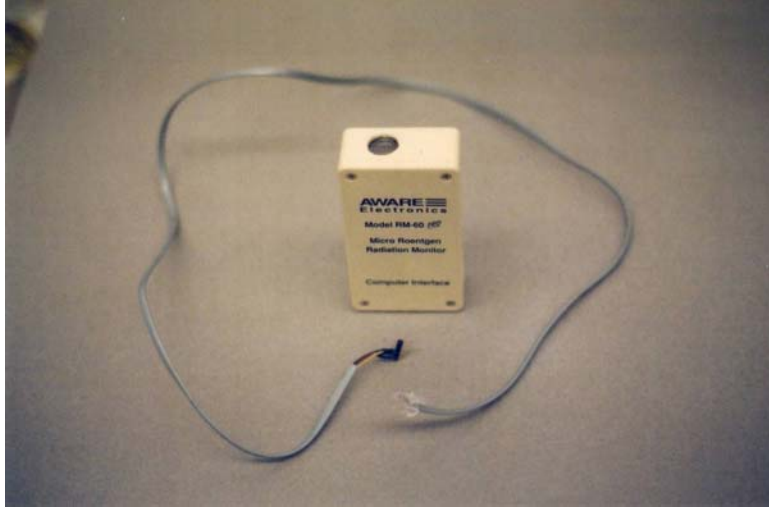
Aware Electronics RM-60 Geiger Counter - The phone cable was modified for my flight computer.
