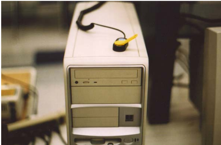
Thermochron Being Programmed – The thermochron is in its reader, sitting on top of the PC.
