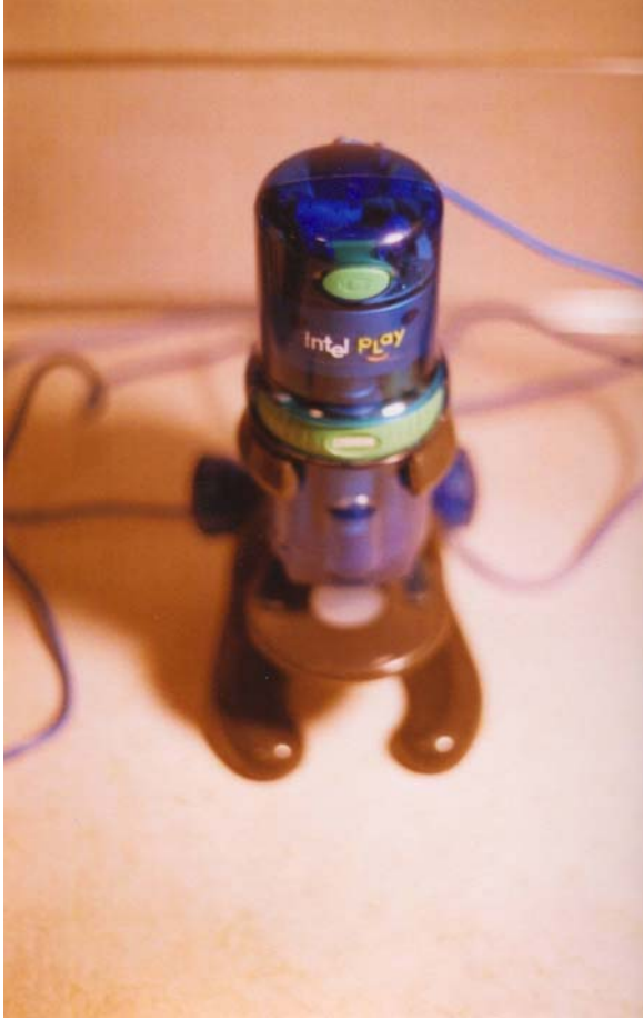
Intel QX-3 Digital Microscope - An easy way to record microscopic images on a PC.
