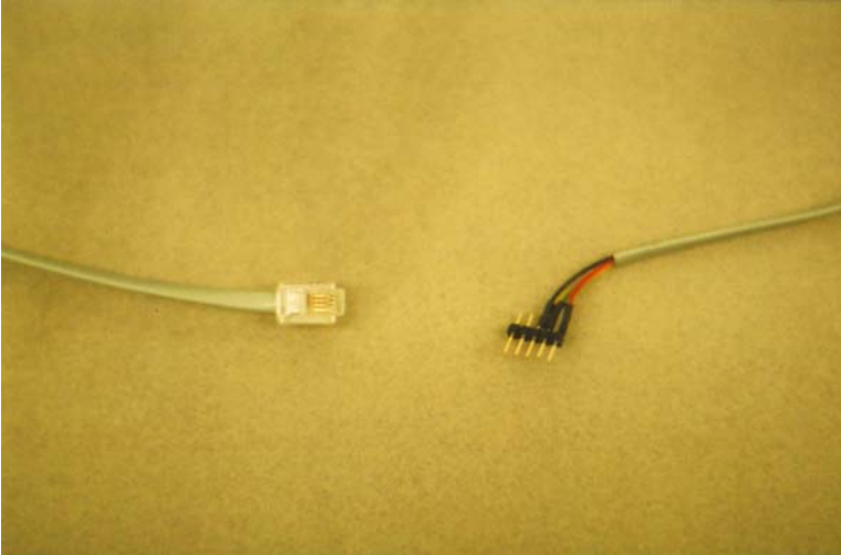
RM60 Cable - Modifying a phone cable (with RJ-11 jack). The black wire of the phone cable is not used.
