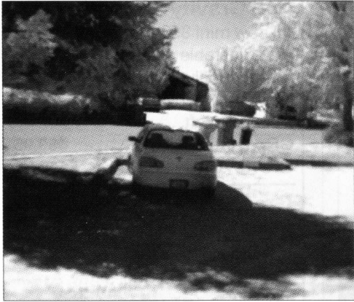
Figure 3. An image with the IR blocking filter removed and the Pencam refocused.
